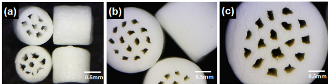
Figure 1. Optical micrographs of different size multichannel granular bone substitutes. (a) 1 mm diameter, (b) 2 mm diameter and (c) 3 mm diameter.
